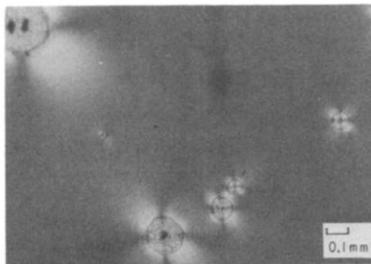
**Figure 6.** Formation of popcorn polymer particles; *m*-bromostyrene with 1.9 wt % *p*-DVB; 144 hours at 70°C.
