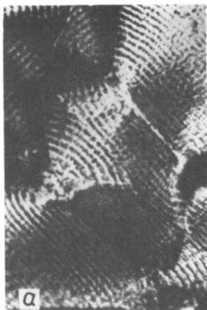
Figure 2. Initial deformation stage of the crack at its center (7)
