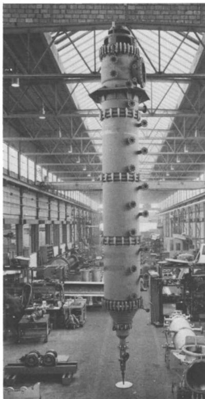
*Figure 10. Industrial size high viscosity machine (Luwa Film-truder) (heating area=12 square meters)*
